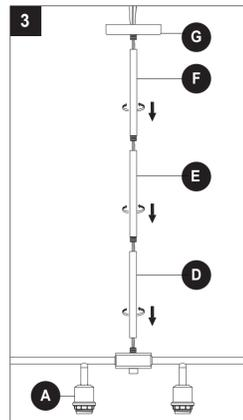
**Note:** To ensure proper assembly, make sure to route the wires through the ends of the rods with the threaded nipple first.
