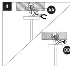
Attach wire nuts (DD) to ends. Tape wire nuts (DD) and wires together with electrical tape (not included).
